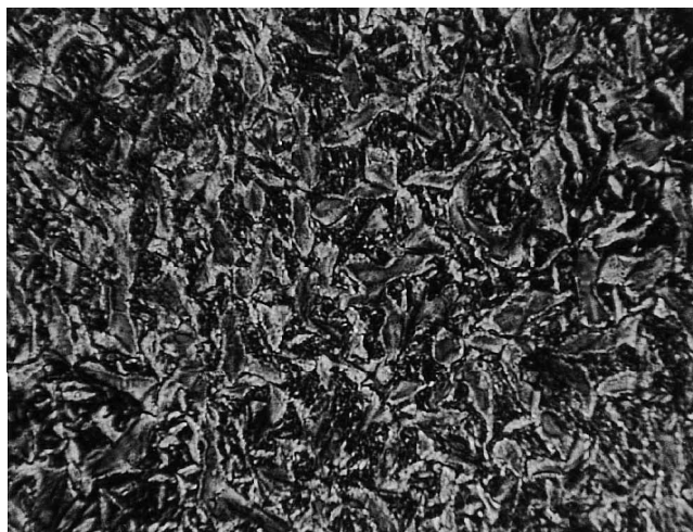
Figure 4. Mesophase texture of LPLCPS ( 250\times ) obtained by polarizing optical microscopy at 100^{\circ}\text{C} .
